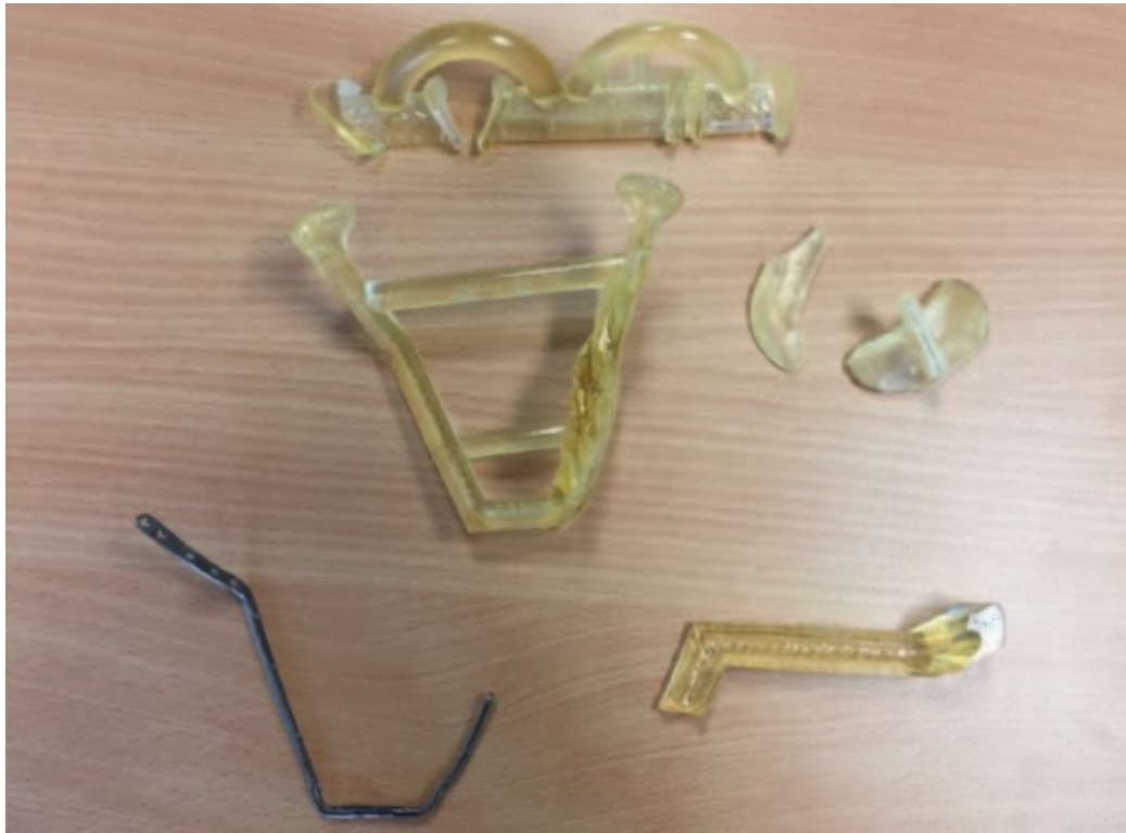
Figure 2. Guided templates, mandibular model, and customized reconstructive plate.
