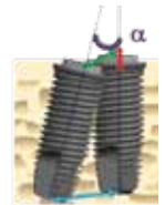
Fig. 2 The accuracy is generally expressed by four parameters: green: deviation at the entry point of the implant or cavity, blue: deviation at the apex of the implant or cavity, purple: deviation of the axis of the cavity or implant, red: deviation in height/depth.
