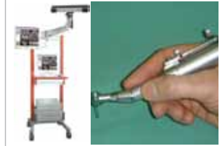
Fig. 12a Navigation system for dynamic surgical guidance. Workstation, graphical user interface, and stereoscopic camera (Courtesy of IVS Solutions AG, Chemnitz, Germany).
