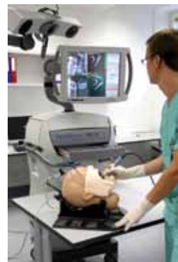
Fig. 14a Dynamic guidance. Simulated implant surgery in dental dummy. For guidance, the surgeon has to look at the navigation screen.
