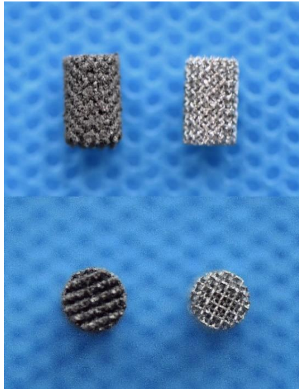
Figure 5.1. WE43 scaffold before (left) and after (right) the chemical polishing.
